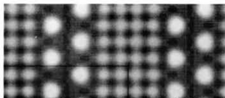
Fig. 4. Synthetic image calculated from the structure model of Fig. 3 by 'multislice' computation for 280 beams through 9 slices of the crystal (thickness 9 \times 3.88 = 34.9 Å). Incident-beam convergence (max. 2.0 \times 10^{-3} rad) taken into account by calculation for 13 beam directions over a quarter of the condenser aperture and summation of the image intensities after symmetry expansion (O'Keefe & Sanders, 1975). Defocus -750 Å; spherical aberration constant C_s = 2.20 mm; focus spread (due to chromatic aberration) = 100 Å; the objective aperture size corresponds to a radius of 0.42 Å ^{-1} in reciprocal space (105–112 beams through the aperture).
